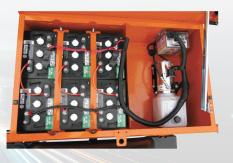
Six 6-Volt Deep Cycle Batteries and hydraulic pump are standard
